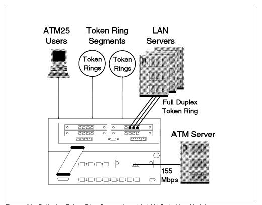
Figure 30. Relieving Token-Ring Congestion with LAN Switching Module
